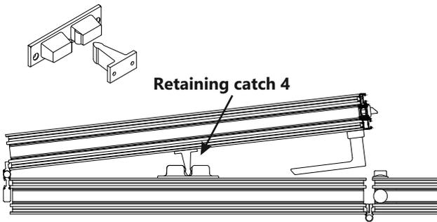
During operation, the panel with an access door needs to be hinged back on to the next panel so the catch engages, before the remaining panels can be folded.
