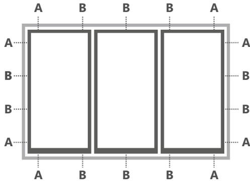
3. Drill holes in the aluminium frame as seen in the figures below. Use 7-10 mm drill bits depending on the screw diameter.
