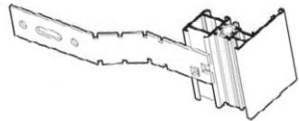
2. Clamp the metal brackets as shown in the figure; 150 mm from the corners (A) and equal distances of max. 800 mm (B) around the frame's sides and top.
